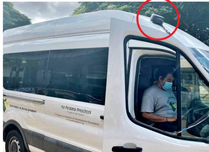
The WiFi on Wheels mobile connectivity unit features a high-speed internet router affixed to the top of a van, which is deployed to various areas around the Wai‘anae community to assist users with connectivity needs.
